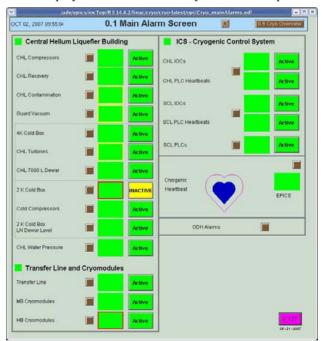
Figure 3: The Cryogenic Alarm Screens existed prior to the new alarm system, and would continue to be required.
