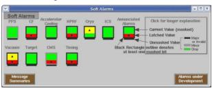
Figure 1: The Top Alarm Summary displays the status of all the alarms in the system. Since EPICS process variables provide the status, the information can be used in any EPICS client application.
