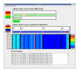
Fig.2 Trend of Beam Loss Distribution shown in MPS Window.
