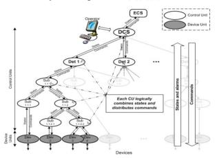
Figure 1: Software architecture.
