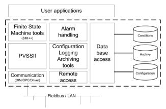
Figure 2: Control system components.
