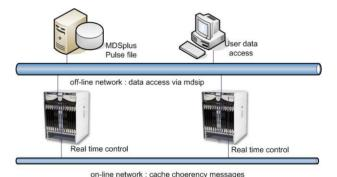
Figure 1: A typical configuration for distributed control.
