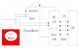
Figure 3: Design of Control Function of Superconducting Devices
