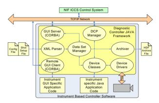
Figure 3: Framework for I-BC software ties instrument applications to ICCS supervisory controls.
