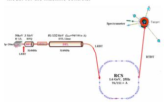
Figure 1: The Schematic Layout of the CSNS Facility
