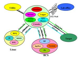
Figure 2: CSNS Controls Scope
