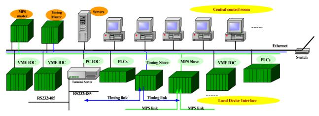
Figure 3: CSNS Controls Architecture
