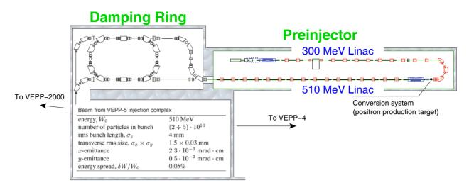
Figure 1: VEPP-5 injection complex layout and parameters.
