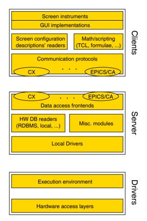
Figure 2: Plugin-based architecture of CX version 4 (shown are pluggable parts).
