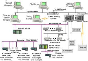
Figure 2: Physical architecture of the NSE control and data acquisition system.
