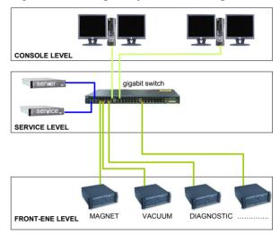
Figure 3: Control System Structure
