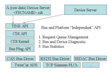
Figure 1: Architecture of the Common Device Interface
