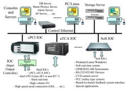
Figure 1: Proposed TPS control system architecture.
