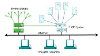
Figure 1:Current System, Showing Centralized Timing and Data Acquisition (RICE)
