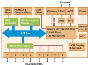
Figure 1: Hardware block diagram of UC7400.
