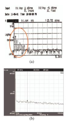
Figure 3: Output current noise spectrum: (a) Old CMPS, (b) Digital CMPS.
