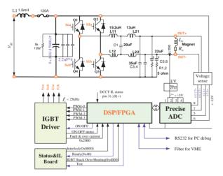
Figure 2: Circuit diagram of the digital control power supply.
