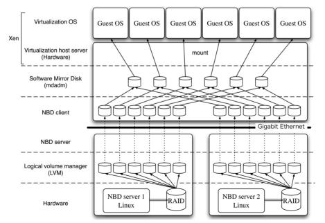
Figure 3: Layout of the Root file system with high availability and high performance.
