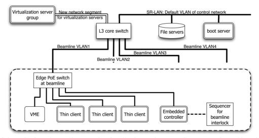
Figure 1 Schematic view of network system for virtualization environment. Components denoted by a double line were newly installed.
