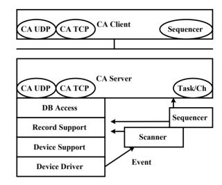
Figure 2: Block diagram of IOC software.
