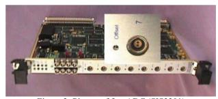
Figure 3: Picture of fast ADC (SIS3301).
