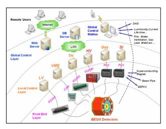
Figure 1: Architecture of the BESIII DCS.
