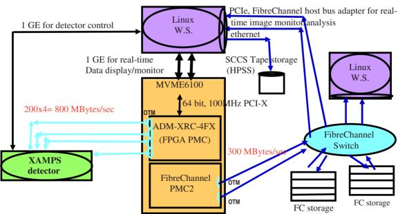
Figure 3: Block diagram of image processing system for testing the XAMPS detector
