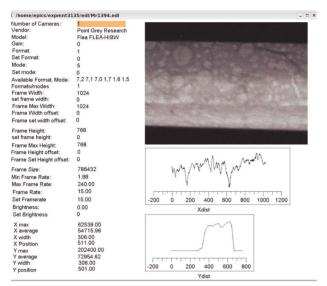
Figure 2: X-ray image of blemishes in the coating of a beryllium window.
