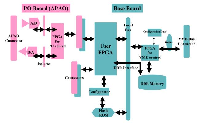
Figure 2: A block diagram of the flexible and logic-reconfigurable VME board. Green blocks are elements on the base board and pink blocks are elements on the I/O daughter board.
