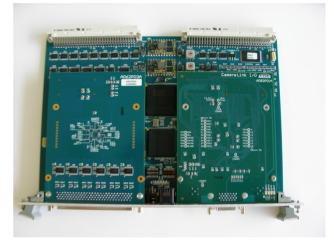
Figure 1: A photograph of the flexible and logic-reconfigurable VME board mounted with DIO (left side) and camera link grabber (right side) daughter boards. The user FPGA (lower) and bus-control FPGA (upper) are mounted in the middle of the base board.
