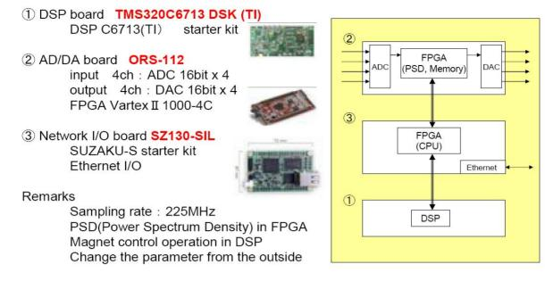
Figure 4: Configuration of the prototype
