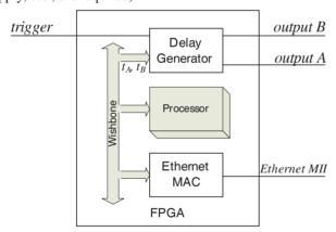
Figure 2: Block diagram of a delay generator.
