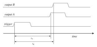
Figure 1: Signals of a delay generator.
