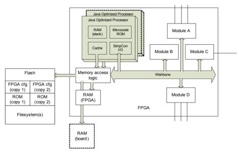
Figure 3: Overview of the hardware architecture.
