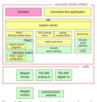
Figure 3: The entire solution is split into two boxes; the controller and power part. The former is placed outside of the tunnel the latter is placed inside. The distance between them is up to 250 m.
