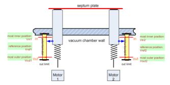
Figure 4: Schematic overview for half of the septum.
