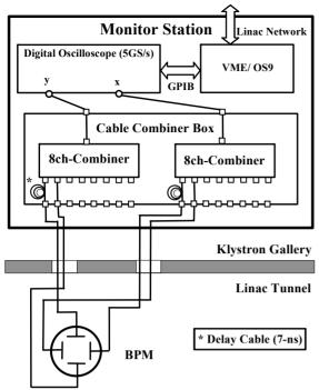
Figure 1: Schematic drawing of previous BPM DAQ system.
