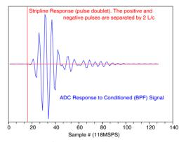
Figure 1: BPM Signal and Typical AFE/ADC Response. On the timescale of the digitizer the pulse doublet (red) cannot be resolved (the LCLS stripline length is  $\approx L = 5 - 6''$ . The band-pass filtered AFE response has a greatly reduced amplitude but is stretched out in the time-domain.
