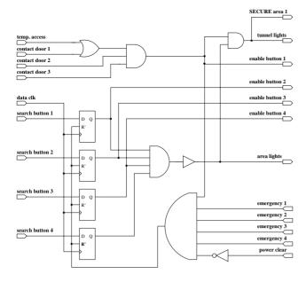
Figure 4: Sample Hardware State Machine (HSM) for One Area
