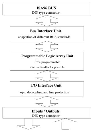
Figure 2: Block Diagram of a Digital I/O Card
