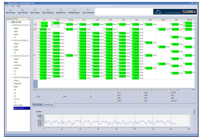
Figure 4: Snapshot of the GUI for the vacuum control of the booster. It has a TauTree on the left, a TauGrid on the top and a TauTrend on the bottom.
