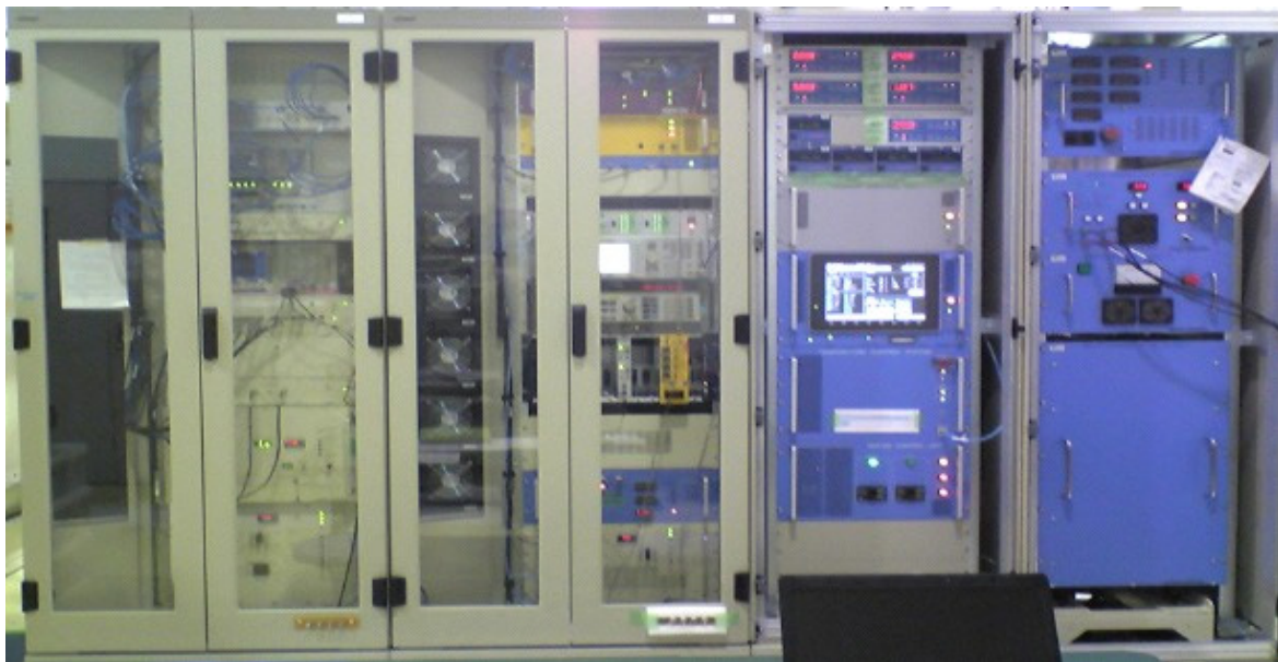
Figure 1: From left to right – rf low-level control units in water-cooled 19-inch rack. The precise water temperature, vacuum, rf high-power systems are located in the two 19-inch racks on the right.
