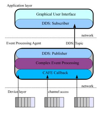
Figure 1: Aggregation of low-level hardware data with CAFE and propagation of summarized data through DDS.
