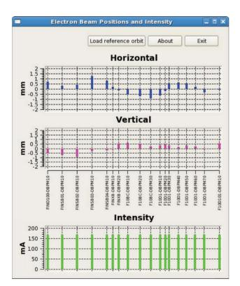
Figure 2: A graphical display of simulated DBPM data built from the Qt (v. 4.3.3) and Qwt (v. 5.1.1) libraries; data are received passively through the assigned DDS Topic. The application is dynamically configured through XML and DDS.
