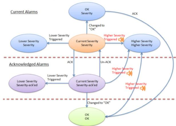
Figure 2: The alarm state diagram for a latched PV.
