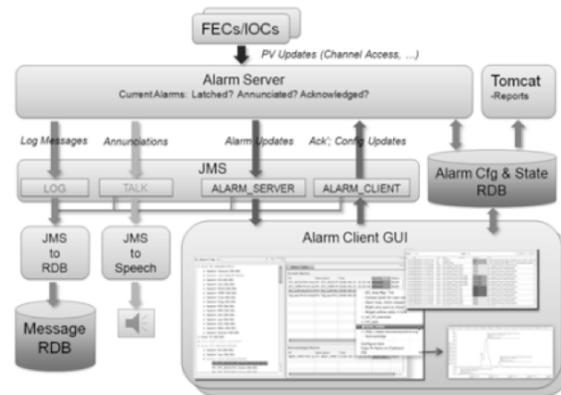
Figure 1: The system architecture of BEAST.
