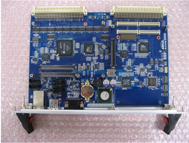
Figure 2: Picture of the COM Express VME carrier board with the remote management daughter card.
