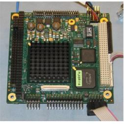
Figure 1: PC/104-plus processor module.
