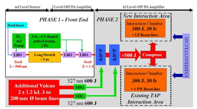
Figure 3: Schematic of the new OPCPA front end oscillator built as an initial proof-of-principle and how it will be integrated into the full system to be built in Phase 2.
