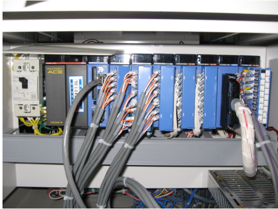
Figure 1: The control system for the new ion source using F3RP61-2L.
