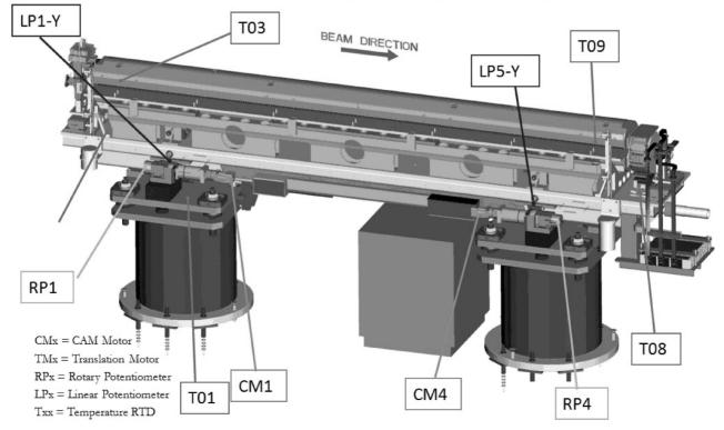
Figure 2: Undulator controls equipment, wall side.
