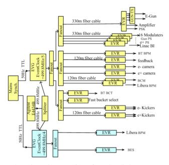
Figure 2: Logic connections of BEPC-II timing system.
