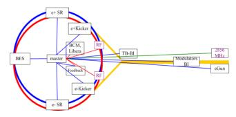
Figure 1: Layout of BEPC-II timing system stations.
