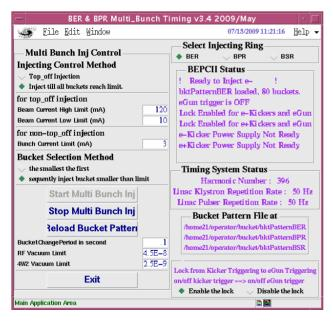
Figure 3: Top-off injection control OPI.
