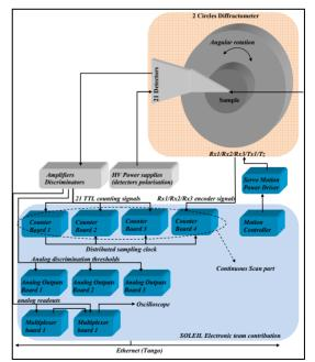
Figure 5: 2 Circle diffractometer architecture overview.
