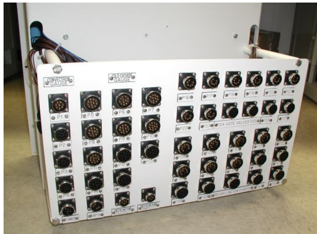
Figure 3: Rear view of PLC interface chassis.
