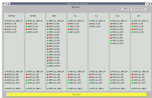
Figure 5: Monitor panel of status for PPS.
