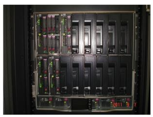
Figure 4: The blade enclosure.
