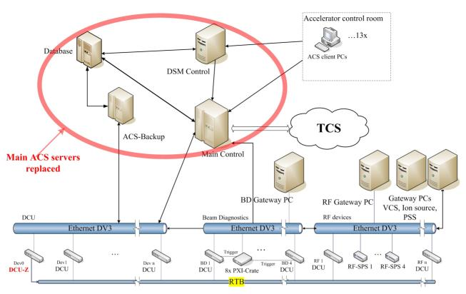
Figure 2: Server architecture and devices of the HIT accelerator control system with replaced servers shown.
