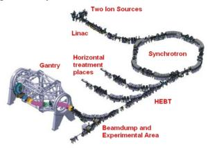
Figure 1: The HIT accelerator facility.
