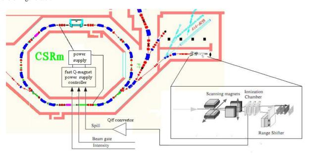
Figure 2: Block diagram of the spill feedback system.
