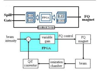
Figure 3: The spill feedback processing.
