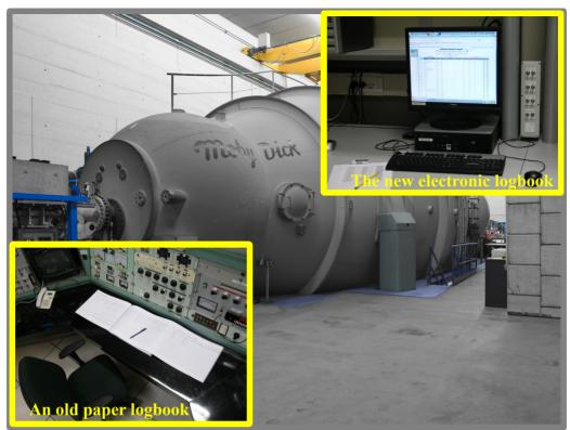
Figure 4: The external tank of the LNL 15 MV Tandem electrostatic accelerator with photos of an old paper logbook and of the new system.
