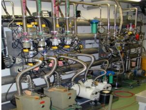
Figure 9: Exhaust gas collecting station.
