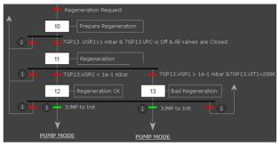
Figure 5: Part of a cryogenic pump process Grafcet (SCADA Panel).
