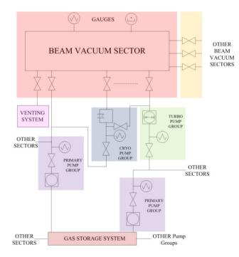
Figure 1: Typical pumps configuration.
