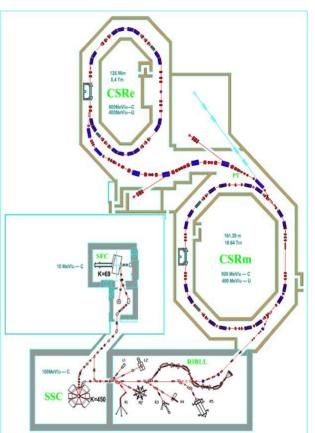
Figure 1: Overall Layout of HIRFL-CSR.
