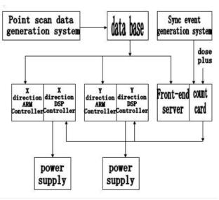
Figure 2: System components.
