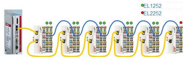
Figure 8: Time resolution test. EL1252 module sends a pulse and all EL2252 measure this pulse and takes a timestamp. The difference of these timestamp is the time resolution of the system.
