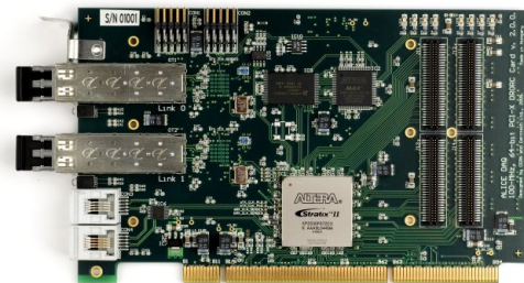
Figure 3: CERN Read-Out Receiver Card (PCI-X slot) with 2 Destination Interface Units.
