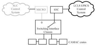
Figure 2: Hardware to enable switch between micro and IOC control.
