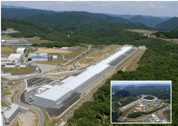
Figure 1: A bird eyes view of the SACLA facility. The electron beams are generated and accelerated from the right hand side to the left inside the linac yard. A picture of SPring-8 site is imposed.
