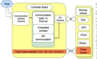
Figure 1: Functional diagram of the SPI BOARD PACKAGE.
