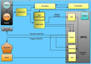
Figure 5: Architecture for PX1acquisition with Pilatus.
