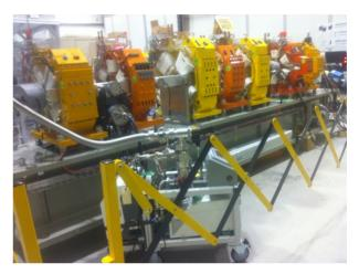
Figure 1: Typical NSLS-II girder assembly
